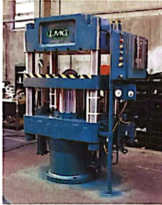
Gambar II.7 Hydraulic press to process desk parts (Tatara, 2017)
