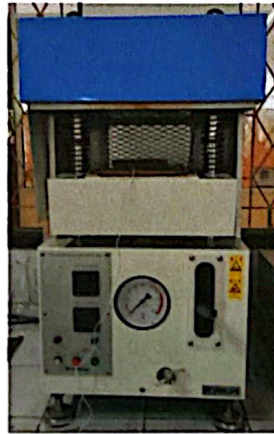
Gambar III.2 Mesin hot press merek Yasuda Seiki Seisakusho
