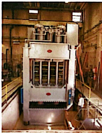
Gambar II.8 Hydraulic press to process thermoplastic fiber-reinforced sheets (Tatara, 2017)
