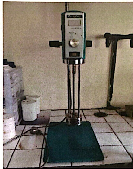
Gambar A.10. High Shear Homogenizer tipe AE 300 LH
