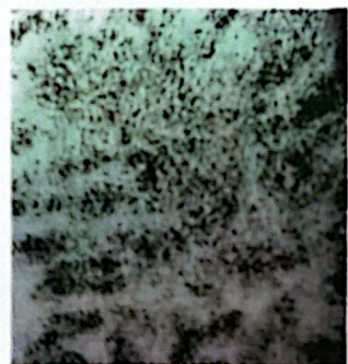
Lembaran Komposit Polipropilena Zeolit 10%wt MAPP 30%wt 185°C
