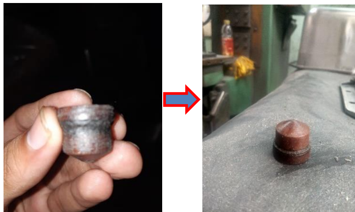
Gambar 5.6 Potensi penggantian pin saat spot welding (Sumber: PT Cidas Supra Metalindo)
