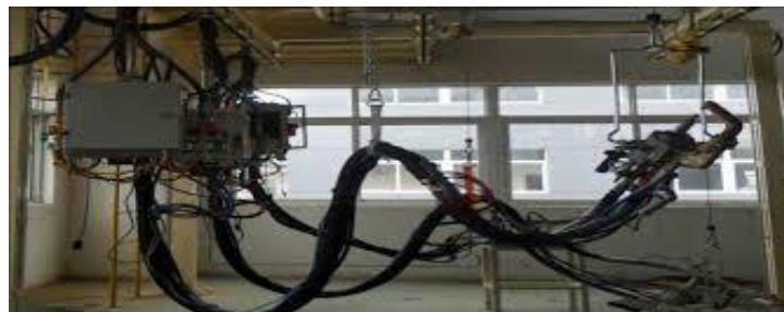
Gambar 4.6 Mesin WPS ( Welding Portable Spot ) (Sumber: PT. Krama Yudha Ratu Motor)
