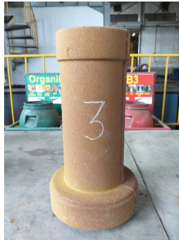
Gambar 4.6 Core BT 1805 (Sumber: PT Bakrie Autoparts)
