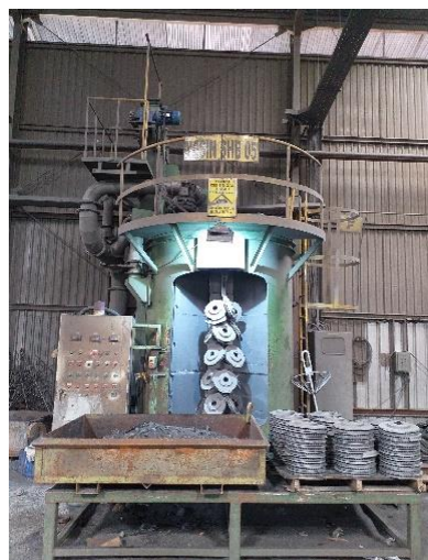
Gambar 4.15 Proses Shot Blast (Sumber: PT Bakrie Autoparts)
