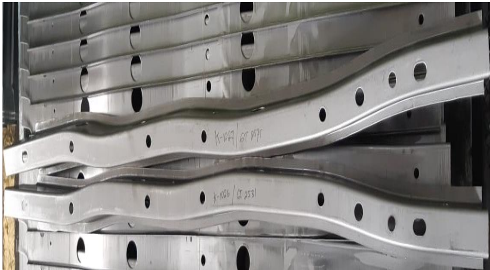
Gambar 4.3 Produk Member RR Side (Sumber : PT Cidas Supra Metalindo)
