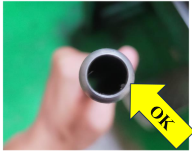
Gambar 5. 6. Hasil OK chamfer headrest Sumber : pengolahan data (2025)
