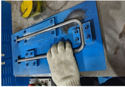
Gambar 4. 12. Pengecekan jig proses bending 2 headrest Sumber : PT Madya Puji Rahayu
