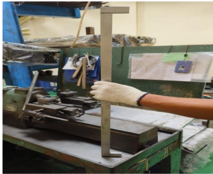
Gambar 4. 7. Jig inspection cutting headrest Sumber : PT Madya Puji Rahayu
